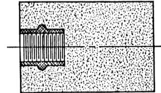
Plugs are a straight cylindrical shape like the diagram right. They have an embedded arbor thread that is available in a number size. The size is expressed diameter x length.
